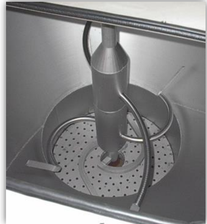
Stirrer and perforated plate bottom to fluidise the sediments
